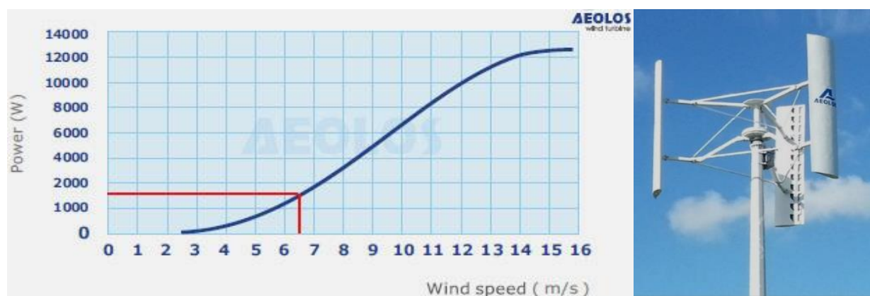
Figure 12: Power curves for 10 KW vertical Axis Wind Turbine [11].
